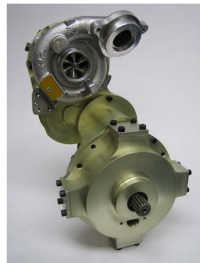
Figure 3: 2 nd generation automotive SuperTurbo
