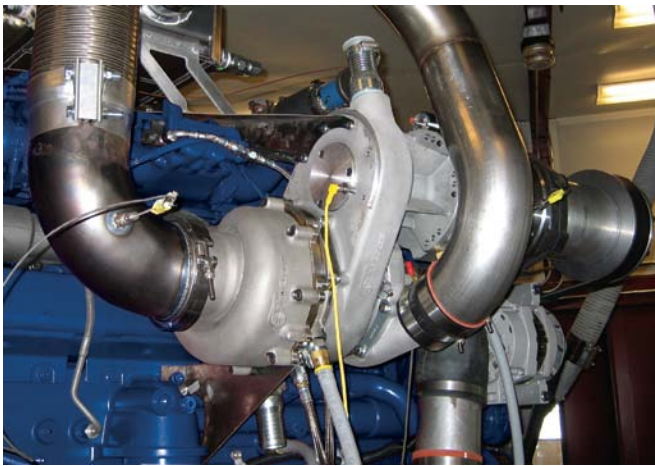
Figure 4: Current generation large diesel SuperTurbo
